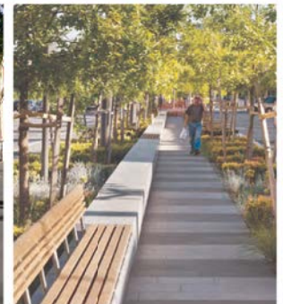
Street furniture integrated with planter walls and edges
